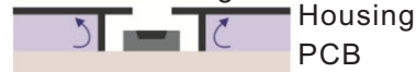
Figure 12: The sensor is isolated from the air inside the housing, which minimizes the impact of the air inside the housing on the sensor.
